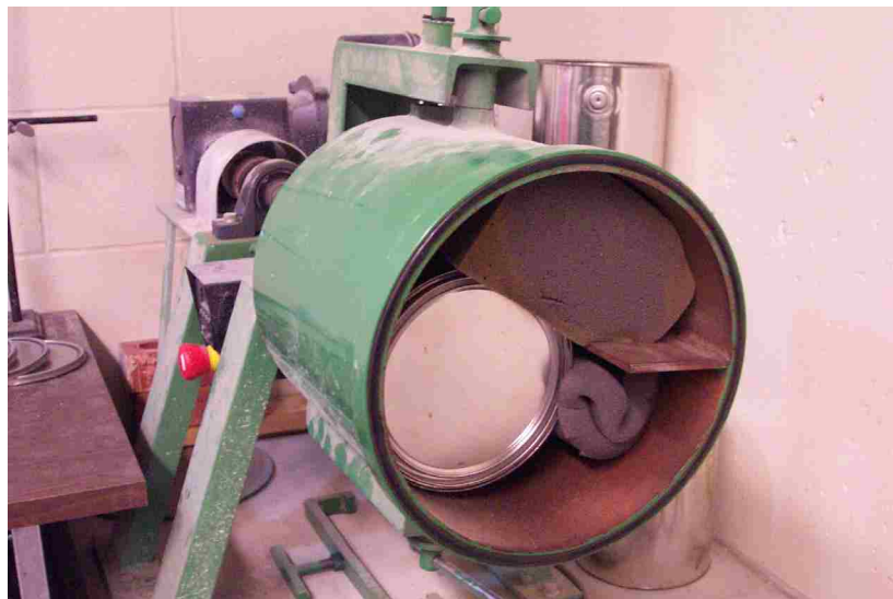
Figure C1. Wet-Ball Mill Device Used For Can Rotation
