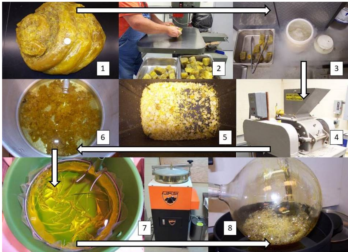
Figure B8. Basic Procedure for RR Extraction and Recovery
